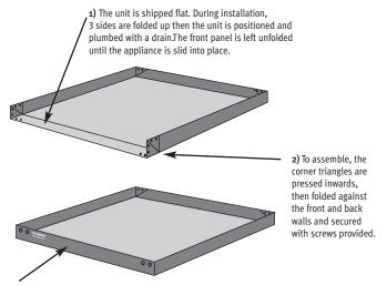
3) After the appliance is in place, the front of the unit is folded up into position and the front panel's screws are installed.
